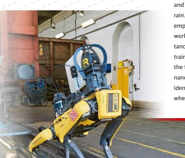
Spot the robot dog goes up stairs, climbs into maintenance pits and safely runs over difficult terrain. This allows it to relieve our employees of physically strenuous work, such as long walking distances or elaborate pit work under trains. In 2023, Spot was used for the first time at a DB Cargo maintenance depot to independently identify freight cars and to inspect wheel set shafts.
